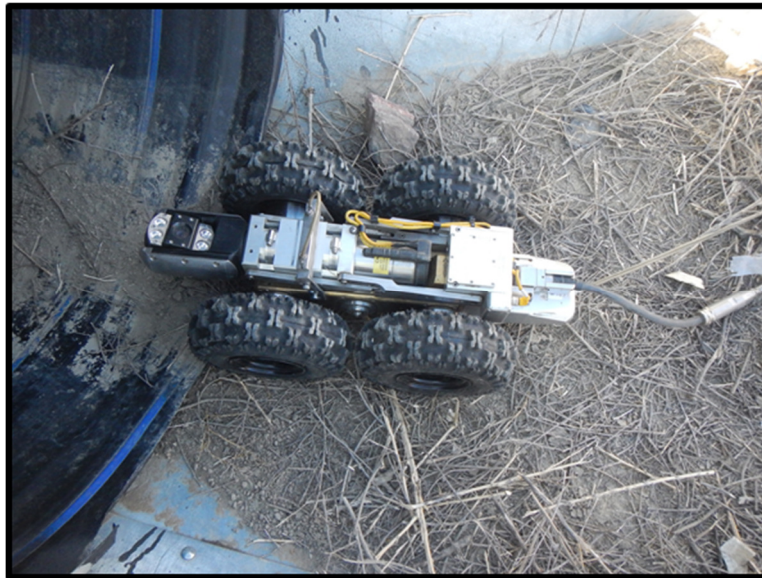
Figure 18. Robotic trolley with mounted, rotatable CCTV camera
